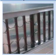
Test specimens are mounted on both the front and back side of the UV Tester, providing a large sample capacity.
